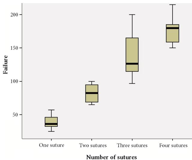
**Figure 5:** A box-plot graph showing the results for the individual suture groups. The  $y$ -axis is failure strength in Newtons.
