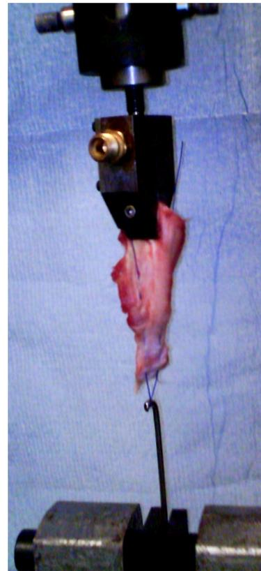
**Figure 4:** The tensile testing setup: the frozen clamp at the top of the tendon, the J-shaped rod attached to the suture loop at the bottom.
