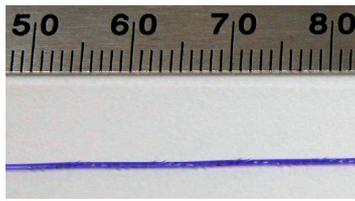
**Figure 2:** A unidirectional barbed segment of the suture (scale: mm)
