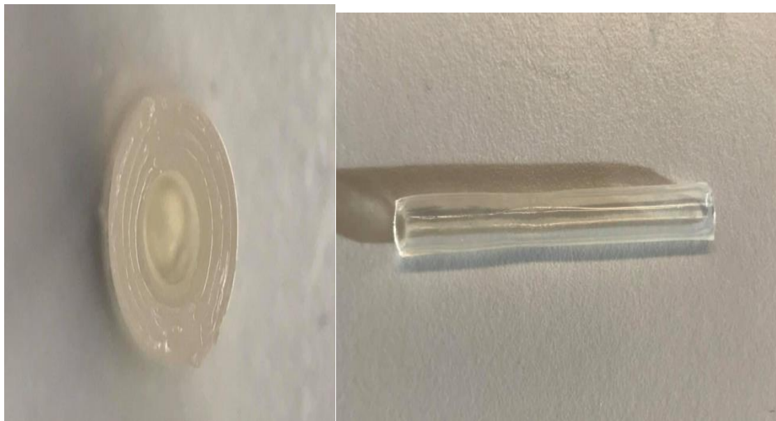
Figure 1: Artificial alginate vessel. The vessel was imaged immediately after fabrication with a simple dip-coating protocol, using 4.4% alginate solution and 200mM barium chloride, with the one base layer and 3 subsequent layer type (A) photographed along its axis (left) and the single 'subsequent' layer type (C) after removal from the dipping rod (right).
