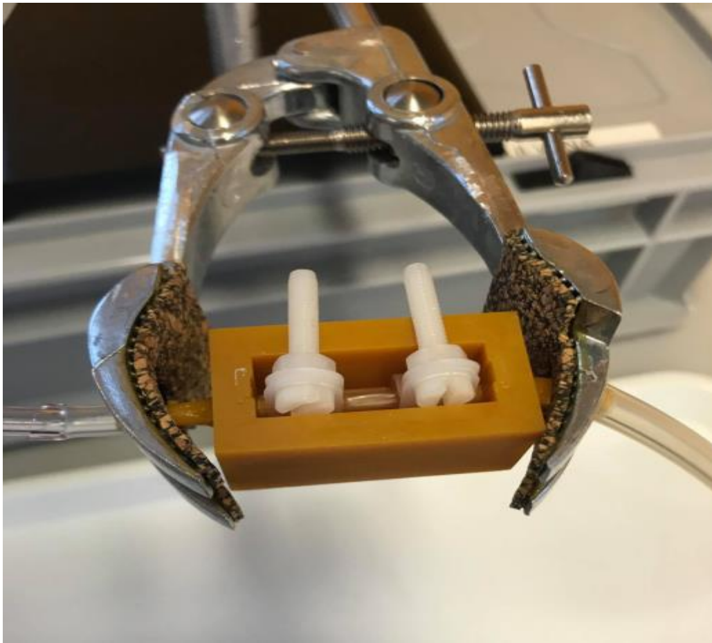
Figure 2: Single layer alginate vessel undergoing 250ml/min perfusion media luminal flow. The vessel is attached to the version two artificial artery in-vitro testing rig via the inner
