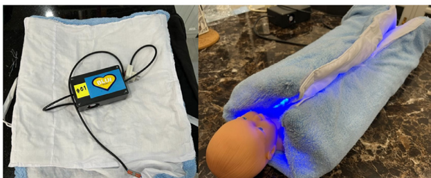
Figure 14: The final product of BLUI blanket PROTO-3
